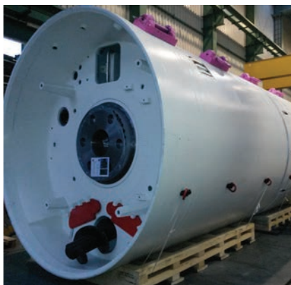
▲ TBM being manufactured in the Herrenknecht factory
